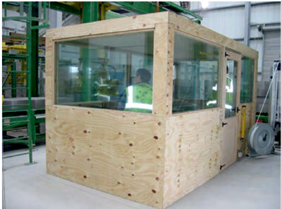
Figure 15 A noise refuge and control room in concrete block manufacturing
