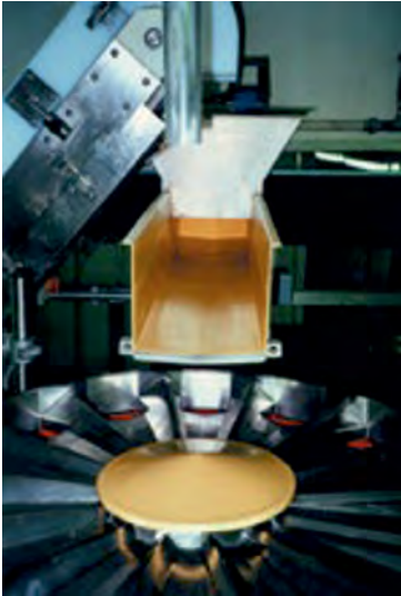
Figure 5 Damping material applied to transport chutes in the food industry
