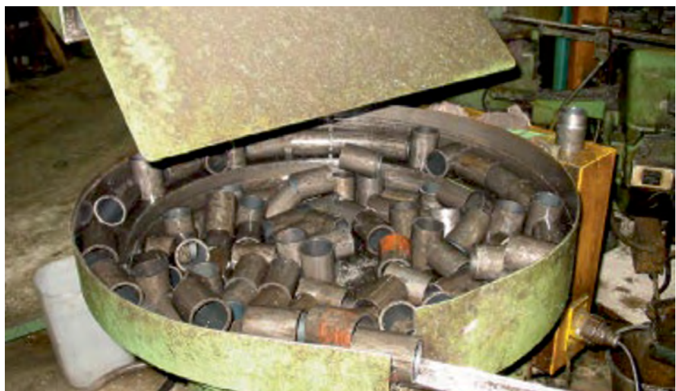
Figure 4 Reduced drop heights to reduce noise
