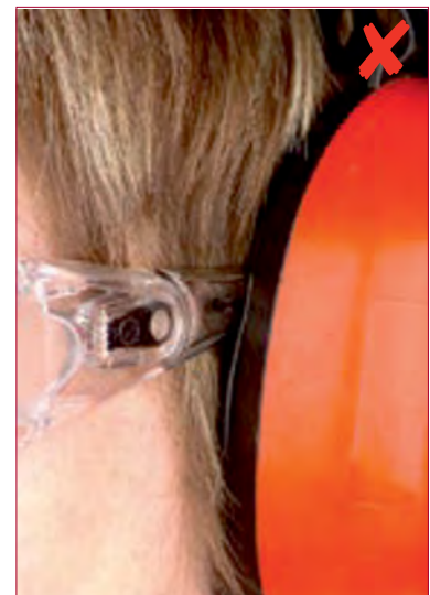
Figure 21 Problems of fitting earmuffs with safety glasses
